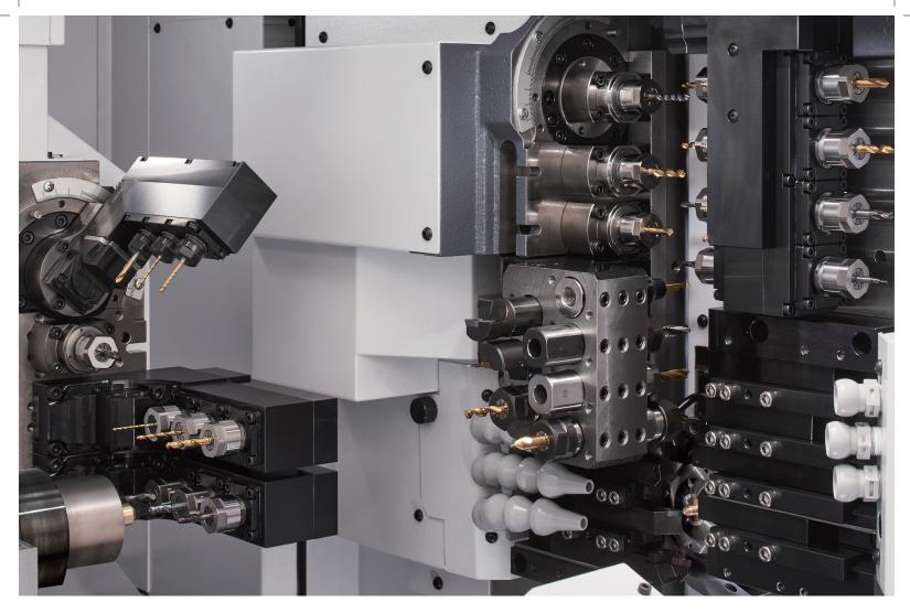
Introducing Citizen's newest development, the D25, equipped with double gang tool posts and B axis. The double gang layout enables short cycle times for high productivity at low part cost. The large number of tools, for both main and sub spindle, gives cost effective production of complex workpieces.
