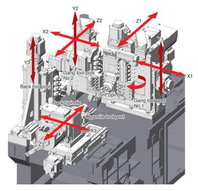
fixed/rotary tools and is equipped with adjustable rotary tool for face, radial or angle machining.
